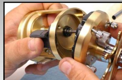
**Important note:** When reinstalling Right Side Plate onto reel, please make sure that the Thumb Bar is held in the “up” position. Otherwise, the clutch will not work.
