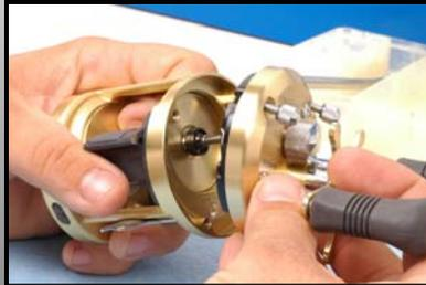
Access the spool assembly on Shimano® Calcutta® and Calcutta B® via thumbscrews located on right side plate. Remove spool assembly
