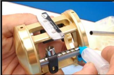
Clean levelwind system of dirt, debris and old grease. Apply 3 drops of Shimano® Bantam® Oil to levelwind. On heavily used reels, Shimano® Drag Grease may be used also be used.
