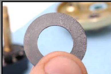
**Lightly** grease drag washers. Too much grease will reduce the maximum amount of grease that the reel will produce.
