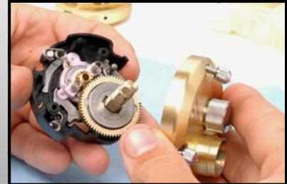
After removal of right side plate screws, remove right side plate.
