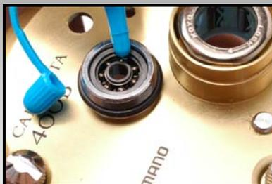
We recommend using only 1 drop of oil on the spool bearing. Excess oil will find its way into the drag system, adversely affecting its performance.
