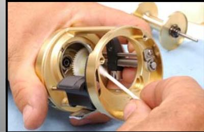
Using cotton swabs and/or a toothbrush with isopropyl rubbing alcohol, clean the exterior of the reel.
