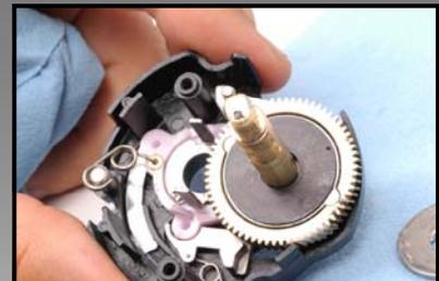
Reinstall drag washer one by one to make sure that they all go in place properly. Handle drag washers with care!
