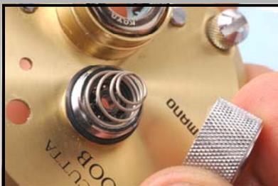
Remove Cast Control Cap. Inspect bearing, spring and O-ring for wear and tear. Clean Cast Control Cap and apply 1 drop of oil.
