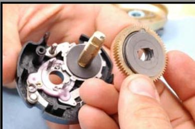
Remove yoke springs, pinion gear, yoke and drive gear with drag washers.
