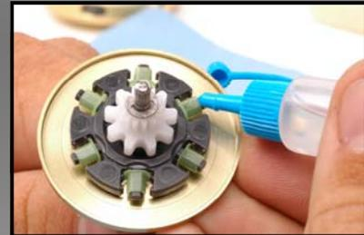
Clean and oil VBS® Brake Collars to maintain optimal casting performance. Inspect collars for wear and tear; replace accordingly.
