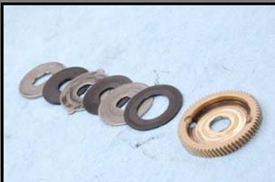
Order of drag washers: Carbon (big hole), metal (keyed), carbon, metal (eared), carbon and thick metal key
