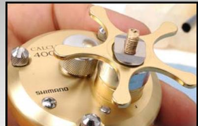
Reinstall star drag, friction washer, handle assembly, handle nut and handle lock plate.
