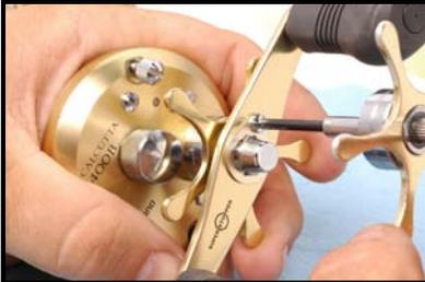
Begin by removing handle assembly using small screwdriver. Thereafter, remove handle nut with 10mm nut driver.
