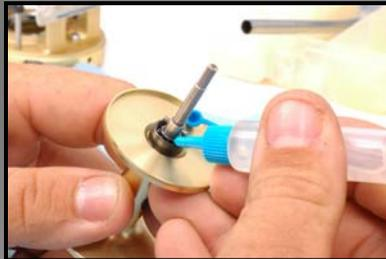
Inspect and clean spool assembly. Check spool shaft bearing or bushing for rust, corrosion or damage. Apply only 1 drop of Shimano® Bantam® Oil to spool shaft bearing or bushing.
