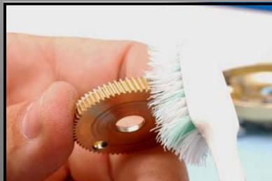
Clean parts with isopropyl rubbing alcohol using a toothbrush and/or cotton swabs.
