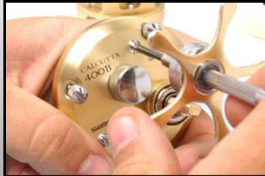
Remove star drag and drag spring washers. Note the order in which the washers are assembled to ensure proper reassembly.
