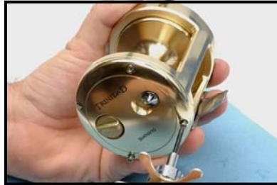
Remove left side plate screws with a Phillips or flathead screwdriver. Take extra precautions to select properly sized screwdrivers to prevent stripping screw heads.
