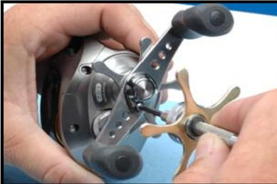
Use a small Phillips or flathead screwdriver to remove handle assembly.
