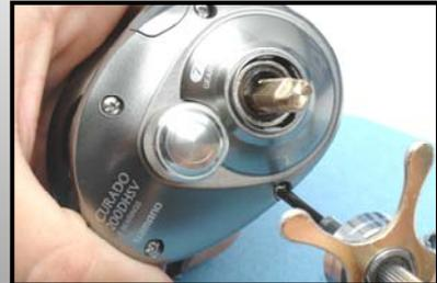
Remove side plate screws. It is always a good idea to lay out the parts in order to aid in reassembly.
