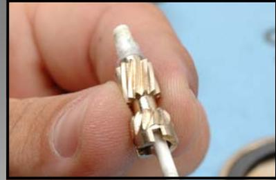
Clean the inside of the pinion gear for optimal freespool performance.
