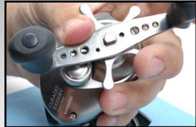
Reinstall star drag, washer, handle assembly. Tighten handle nut with 10MM nutdriver or wrench.
